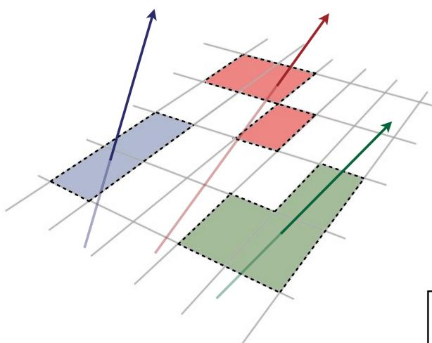
Position of crossing is computed from the signal heights inside the cluster of pixels:
