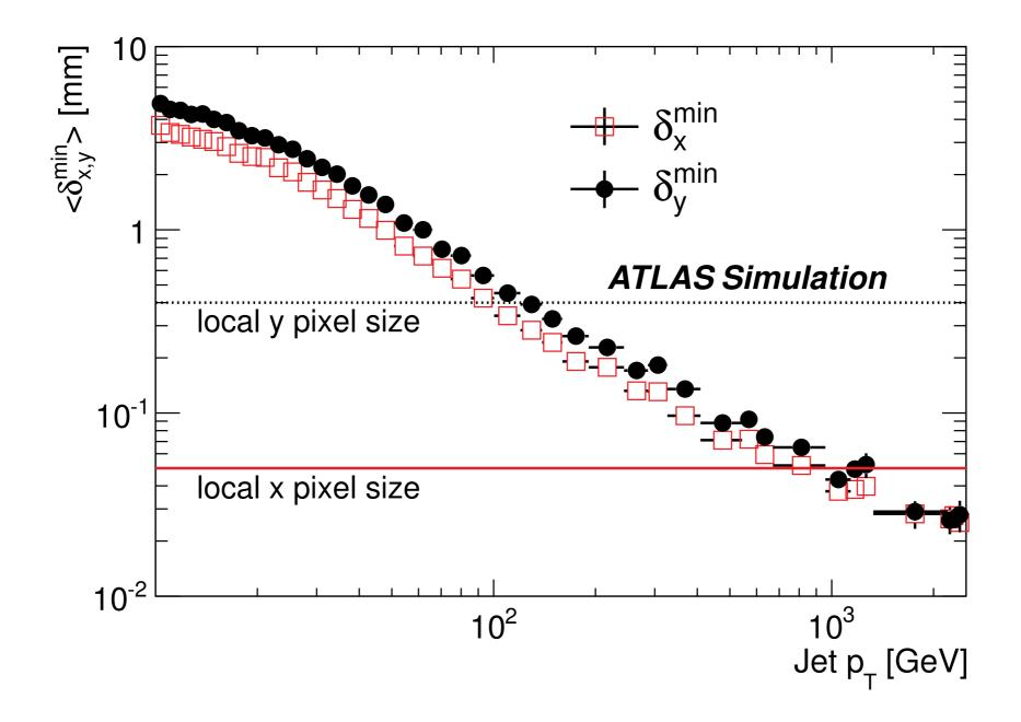
**Figure 4.** Average separation between the two closest charged particles in a jet in the transverse ( $<\delta_x^{min}>$ , open squares) and longitudinal ( $<\delta_y^{min}>$ , full circles) direction at the innermost layer of the pixel barrel. This is shown as a function of the transverse momentum of the jet. The pixel size in the transverse (50  $\mu$ m) and longitudinal (400  $\mu$ m) direction is indicated with the solid and dotted lines, respectively.
