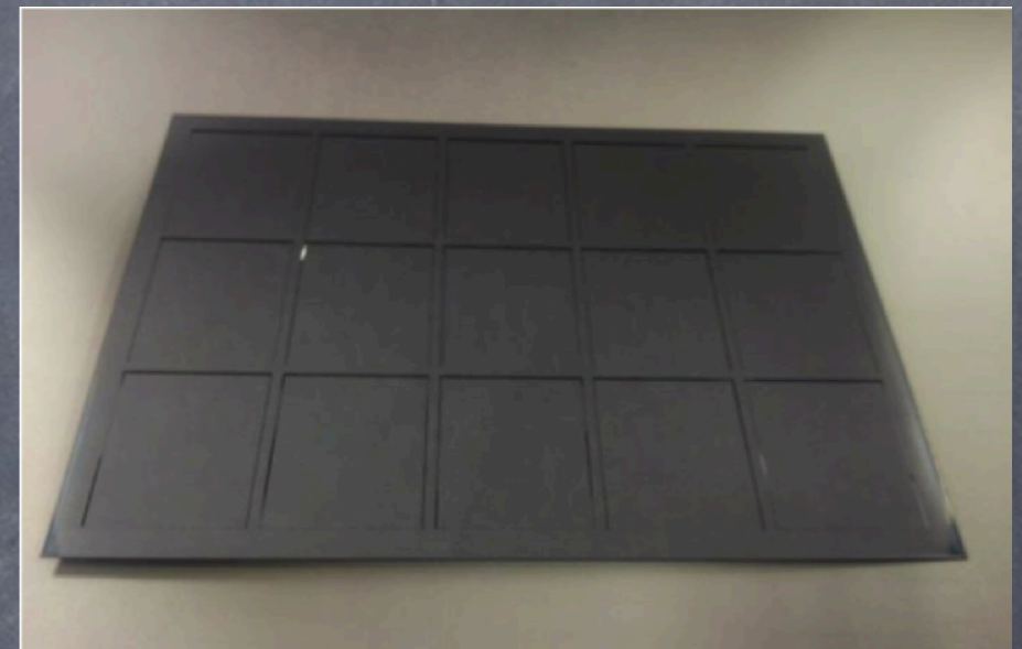
Prototype of the silicon sensor with support ribs and 5x3 cm 2 thinned areas.
