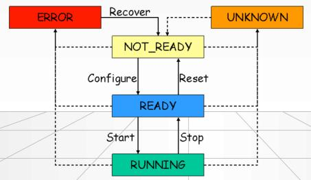
LHCb DAQ /Trigger Finite State Machine diagram (simplified)
