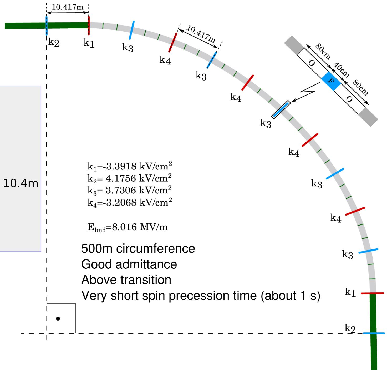
$$\begin{aligned}k_1 &= -3.3918 \text{ kV/cm}^2 \\k_2 &= 4.1756 \text{ kV/cm}^2 \\k_3 &= 3.7306 \text{ kV/cm}^2 \\k_4 &= -3.2068 \text{ kV/cm}^2\end{aligned}$$
