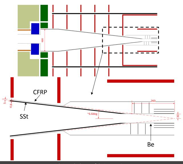
Vertex detector closed air/N<sub>2</sub> circuit
