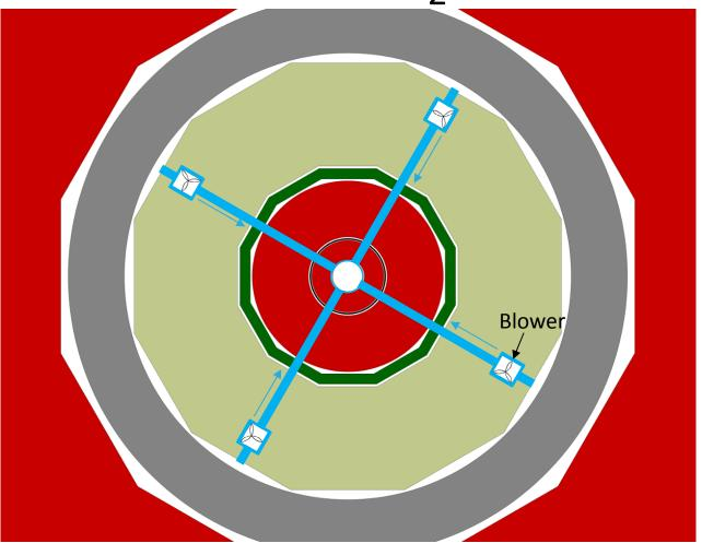
The cross-sectional area of the air duct at the largest diameter of the beampipe (7500 mm<sup>2</sup>) is equivalent to 4 25x75 mm<sup>2</sup> ducts.
