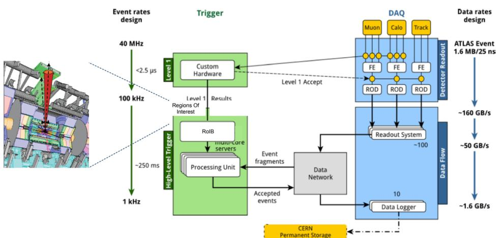
In this readout architecture, the RoIB guides the HLT by building an event fragment with the RoIs used by the HLT to retrieve partial information from the Readout System (ROS) and thus eliminating the need to make a trigger decision based on the full detector readout which will be technically challenging and expensive at high rates.
