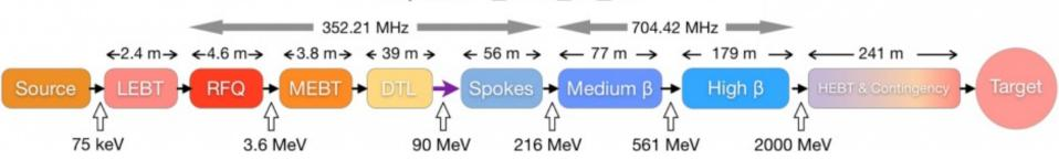
After the DTL, the energy of the proton beam is 90 MeV. In case of a beam size of 2 mm radius/and direct impact, melting would start after about 200  $\mu$ s. Inhibiting beam should be in about 10% of this time.
