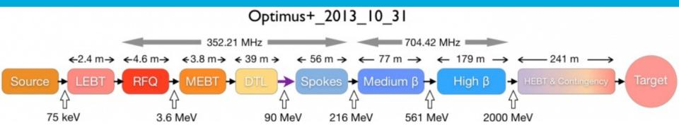
Pulsed neutron source, consisting of a 600 m long LINAC, a spallation target and 22 neutron beamlines
