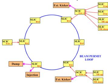
SLIC (SPS Local Interlock Controller) is now a standard BIC.
