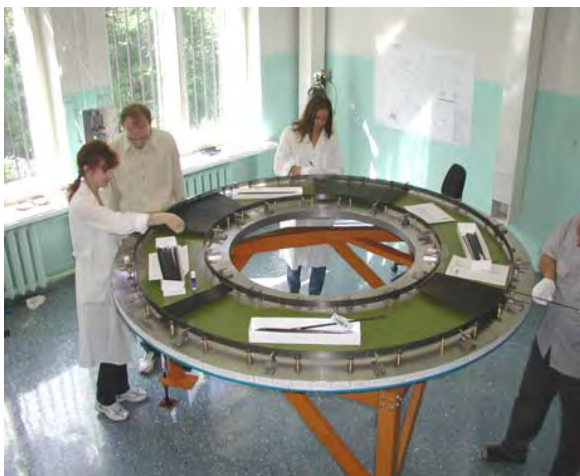
Installation of straws (tests leak tightness)
