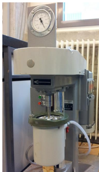
TiC + Carbon Black - Milling and mixing
