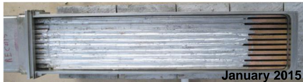
Staggered ends soldered in grooves machined in copper blocks
