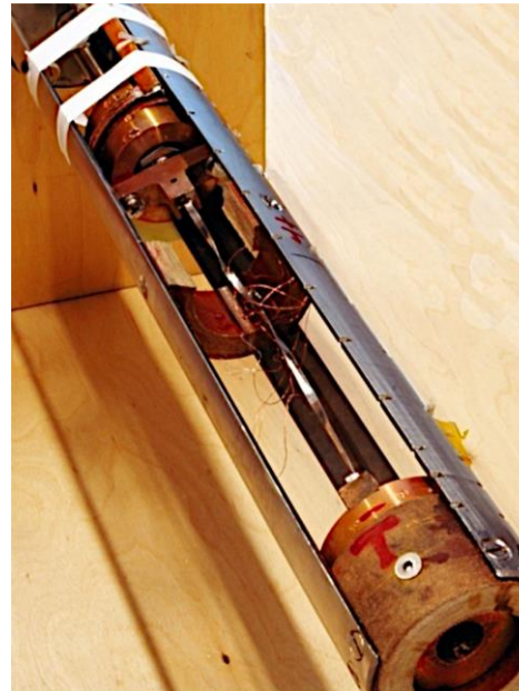
Combined controlled torsion + tensile axial stress
