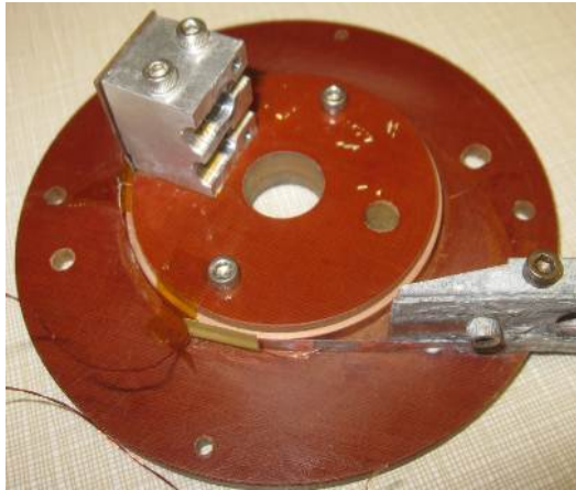
No-Insulation REBCO pancake coil
