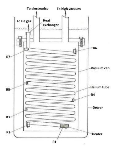
Transient T-development of Hell in an adiabatic walled pipe, open to He bath at one end and heated at the other.
