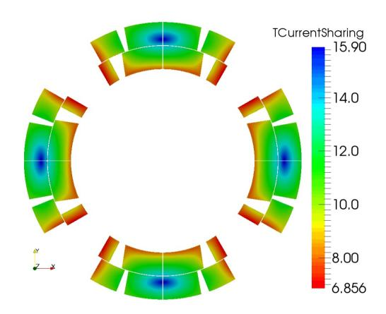
This current sharing map, based on a 1.9 K coil temperature, has now to be combined with the calculated T-distribution due to the heat loads (see next slides)
