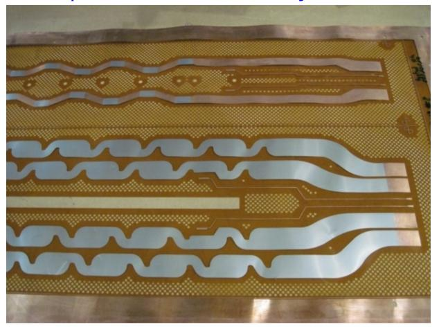
Perforated quench heaters, glued on inner coil layer, facing the helium annulus
