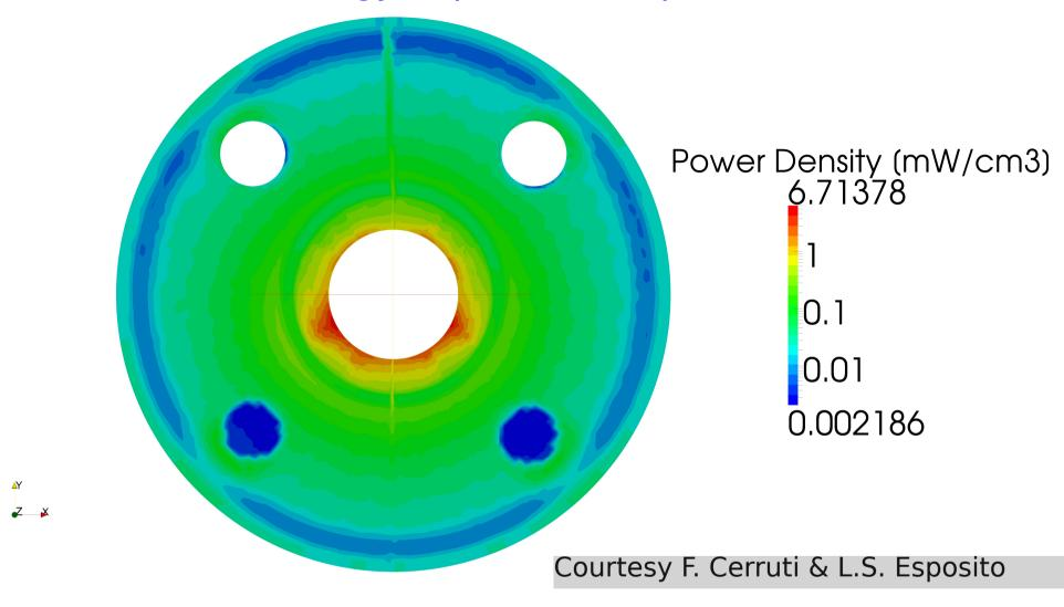
Highest power density in the inner coil layer ~ 7 mW/cm<sup>3</sup>
