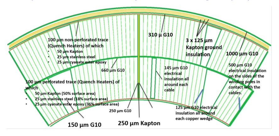
Nb<sub>3</sub>Sn coil block showing all materials used
