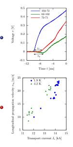
The propagation velocity was measured with the Time-of-Flight (ToF) method, using the voltage waveform along one or three consecutive coil segments.
