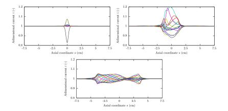
View of the strands adimensional currents along the cable at  $T_0 = 4.2$  K,  $I_t = 14$  kA. Above, left: t = 0.3 ms, above, right: t = 1 ms, below: t = 2.5 ms after the disturbance.
