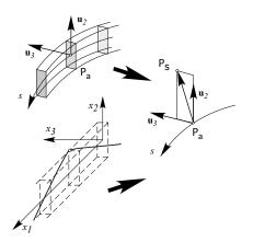
In THELMA, the SC cable is a 3D object characterised by its curvilinear axis, around which strands are built:
