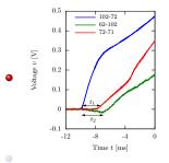
The propagation velocity was measured with the Time-of-Flight (ToF) method, using the voltage waveform along one or three consecutive coil segments.
