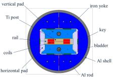
Short racetrack coil made with Nb<sub>3</sub>Sn, developed in the frame of the Next European Dipole Joint Research Activity.
