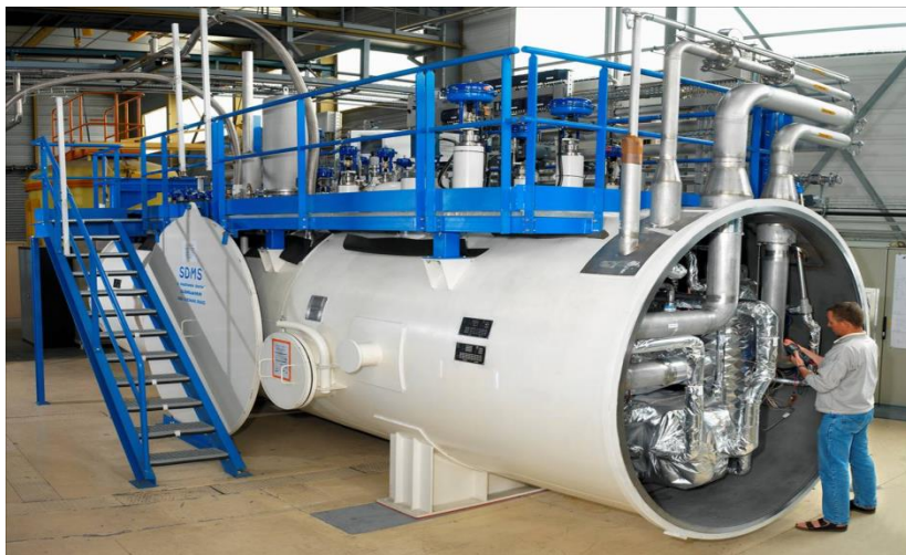
INAC/SBT refrigerator – 400 W at 4 K
