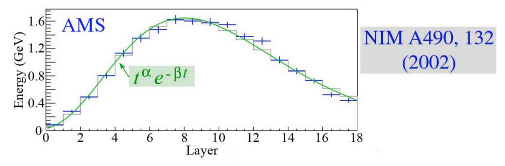
Pb/scintillating fiber 18 layers (17 X<sub>0</sub>)
