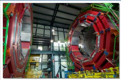
Barrel Muon System
