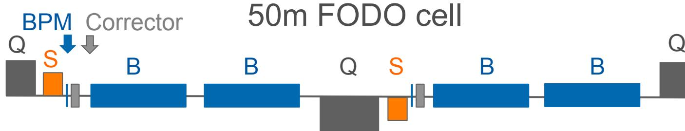
B = bending magnet, Q = quadrupole, S = sextupole
