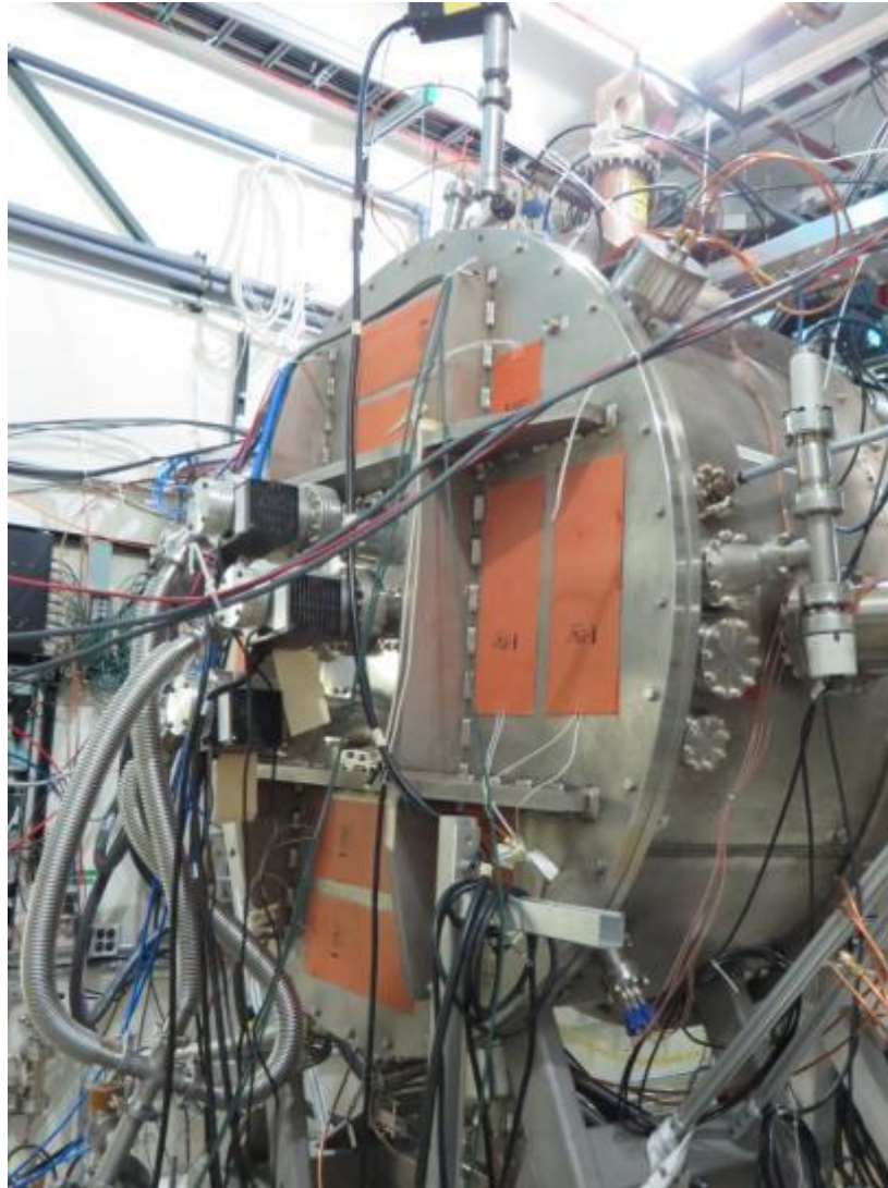
Singe Cavity Test Stand during tests at FNAL
