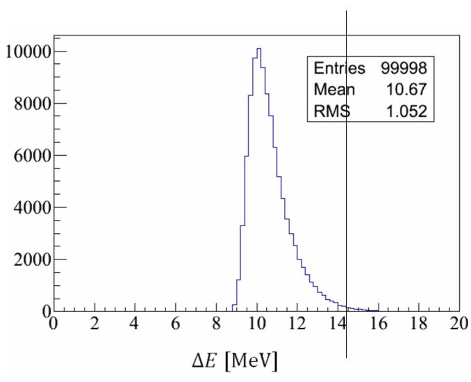
Simulated Energy loss distribution for 200MeV muons in 35cm LH2.
