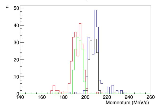
Blue – US reconstructed MC.Mean = 208.475 MeV/c, RMS = 6.252Red – DS reconstructed MC.Mean = 191.643 MeV/c, RMS = 6.430Black – US MC dataMean = 207.263 MeV/c, RMS = 3.249Green – DS MC dataMean = 193.546 MeV/c, RMS = 3.251
