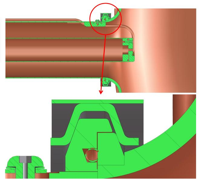
The coupler flange will have a lip to capture the cavity flange
