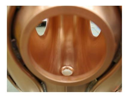
Inner surface finish of the first EPed MICE production cavity at LBNL (photo taken on 2/21/2015)
