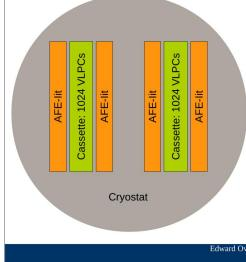
Each cryostat contains two "cassettes", and has 2048 channels of readout
