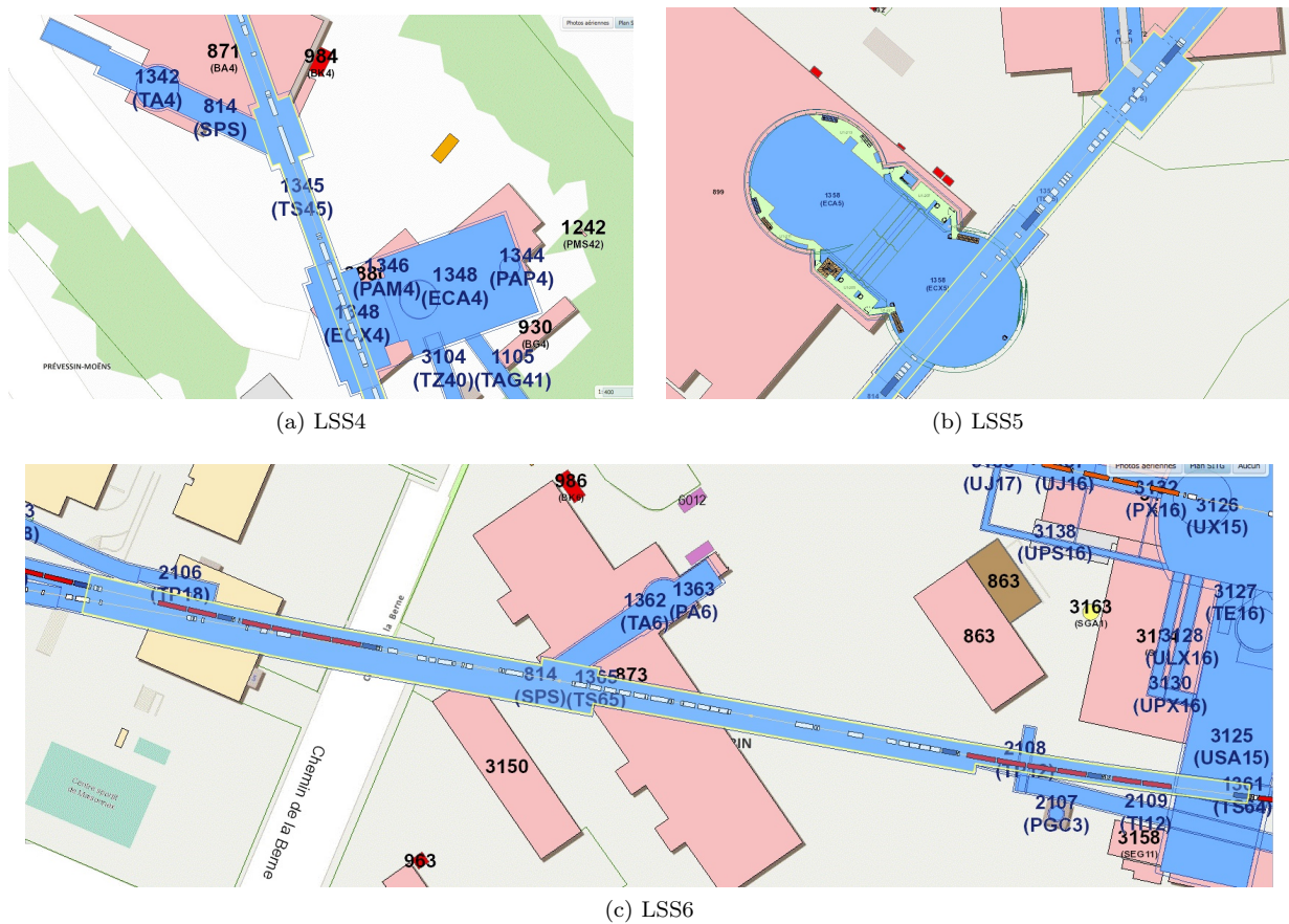
Figure 3: Breakdown of SPS LSS locations where a crab cavity installation could be installed. Tunnel and underground areas shown in blue, and surface buildings shown in pink. The possible locations for a crab cavity installation are where there is at least a 10m section of available beam line space in a section of tunnel that is larger than the standard arc sections.
