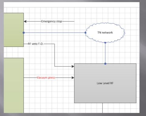
Standard fast interlock to Switch and protect LLRF module fiber optic link
