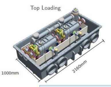
Proposed SPS cryomodule with 2 Crab Cavities. The cryomodule is designed to accept all three CC makes
