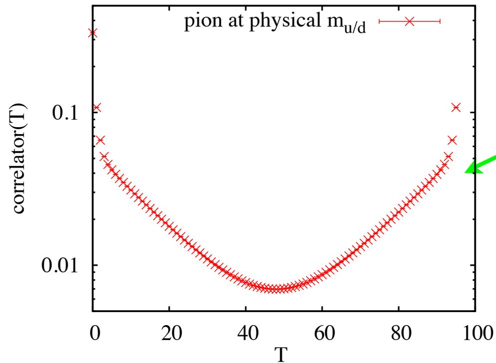
Extract meson mass and amplitude=decay constant from correlator for multiple lattice spacings and  $m_{u/d}$ . Very high statistics
