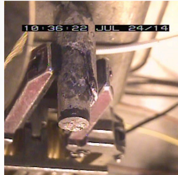
High-resolution video capture of a zircaloy-clad fuel rodlet with Pb-Bi eutectic on the exterior, held in manipulator fingers
