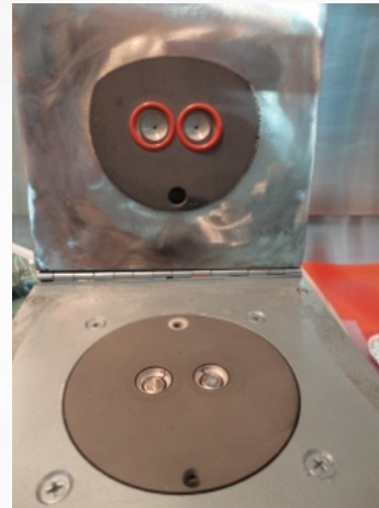
Specific Heat via DSC Perkin Elmer Pyris 1
