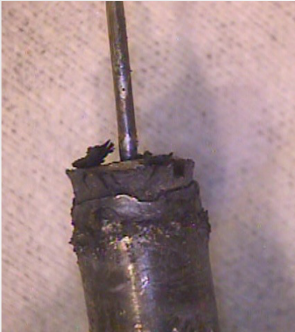
High-resolution in-cell photograph of failed fuel rodlet with centerline thermocouple
