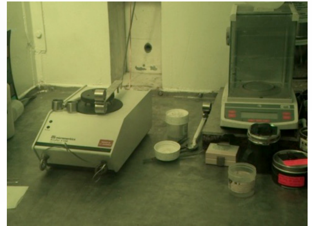
Density via He Pycnometry Micromeritics AccuPyc 1300
