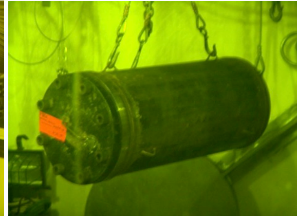
Positioning Loaded Container for Removal from Hot Cell
