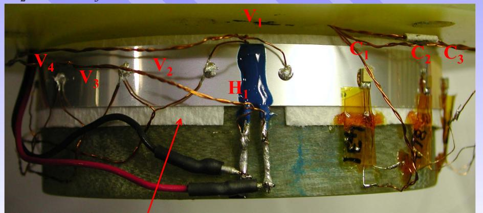
paper to accommodate thermal contraction and reduce conduction to G10
