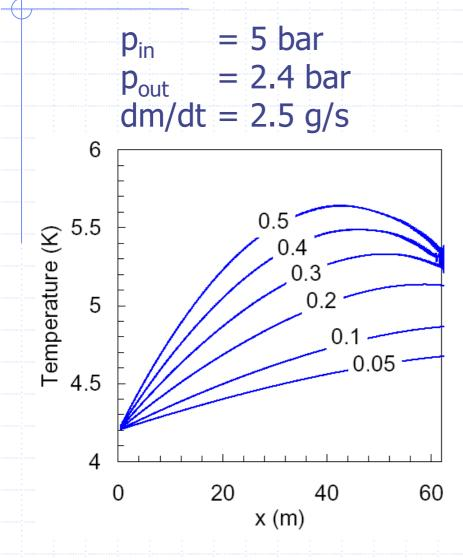
♦ maximum temperature is inside the coil for high heat load (above 13 W/coil) because of JT expansion along the cable
