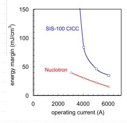
analysis of stability margin as a function of the operating current simplified simulation supercritical helium at 3 bar, 4.22 K no transient heat transfer 1 ms perturbation time
