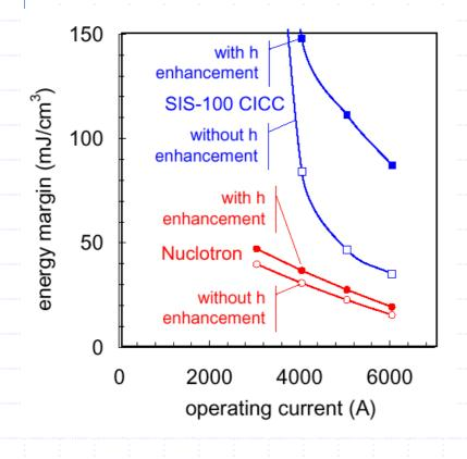
effect of transient heat transfer important ! model as a boundary layer diffusion supercritical helium at 3 bar, 4.22 K 1 ms perturbation time gain in stability is exceptional: a factor 4.5 from 20 to 90 (mJ/cm<sup>3</sup>)
