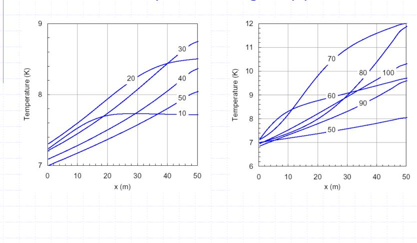
Temperature distribution among the pipes differences in friction factor +/- 15 %
