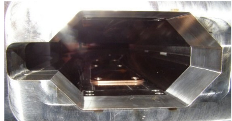
Biased electrodes at DAΦNE, Italy
