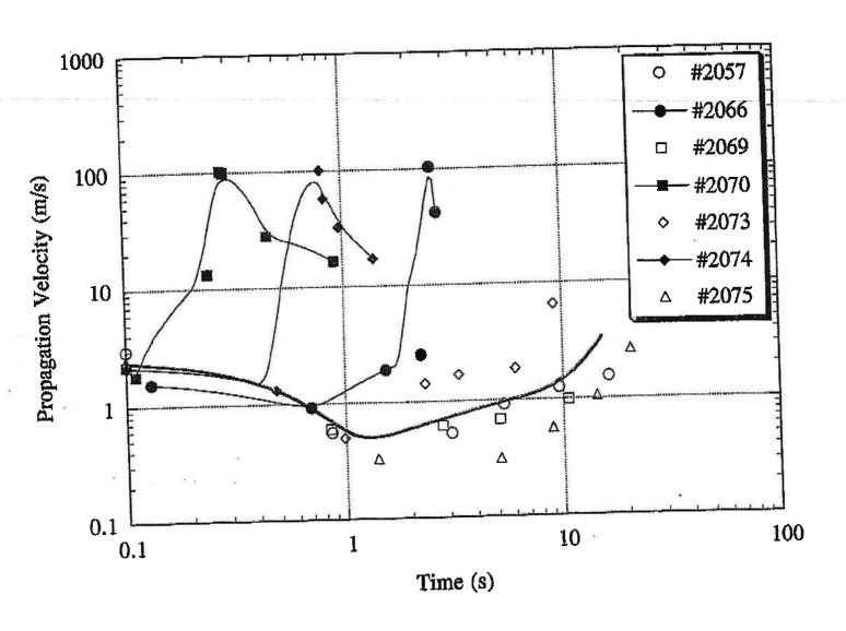
When THQ existed, transient velocities of more than 100 m/s were observed. The sonic velocities were about 130-150 m/s under the present helium test conditions. For shots without THQ there was a trend of slowing down in the hot helium expansion velocity before a gradual increase took place.
