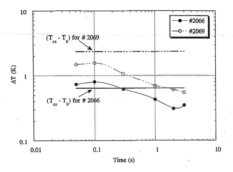
Calculated Temperature Rise in Cold Helium in Comparison with the Current Sharing Margin for a Shot with THQ and one without THQ. This was done with the technique of Dresner's IEEE '89 paper.
