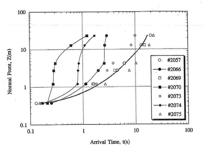
Sharp increases in normal front propagation were observed for shots #2066, 2070, and 2074. A single line was drawn through the other shots that showed the general trend of gradual increase in propagation.
