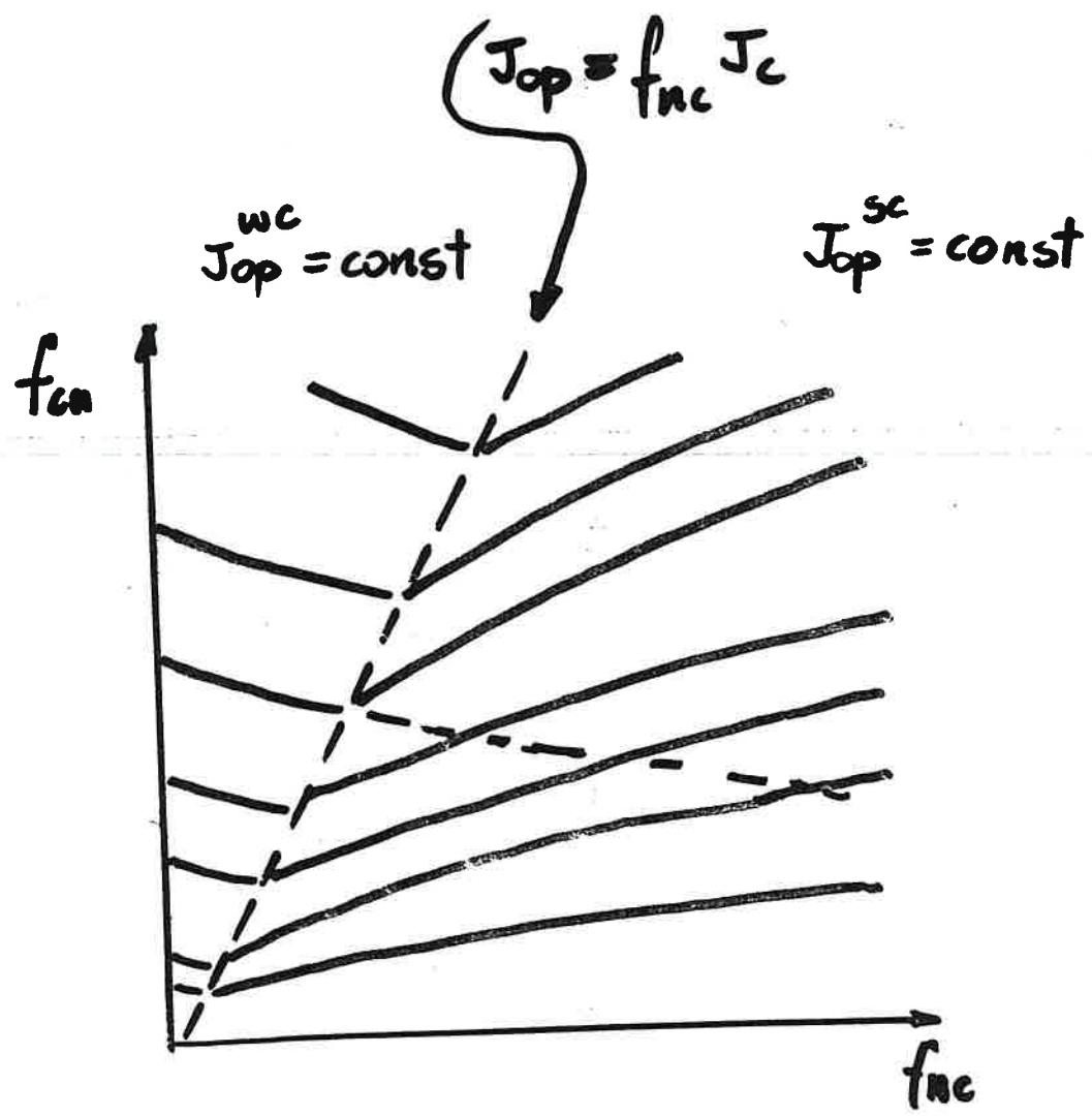
$$J_{op} = \cos \theta \quad \frac{4K_p}{\eta d} \quad \frac{\rho (T_c - T_{op})}{J_c} \quad \frac{f_{cu} (f_{cut} + f_{uc})}{f_{uc}}$$
