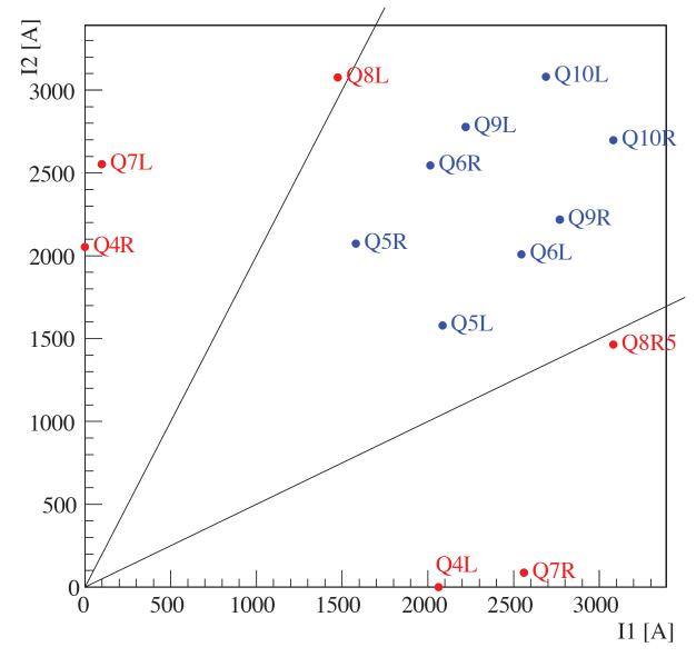
3 magnets each left and right outside the ratio 2 limits, for Q4, Q7 by a lot: Over 2000 A on one beam and close to zero on the other beam
