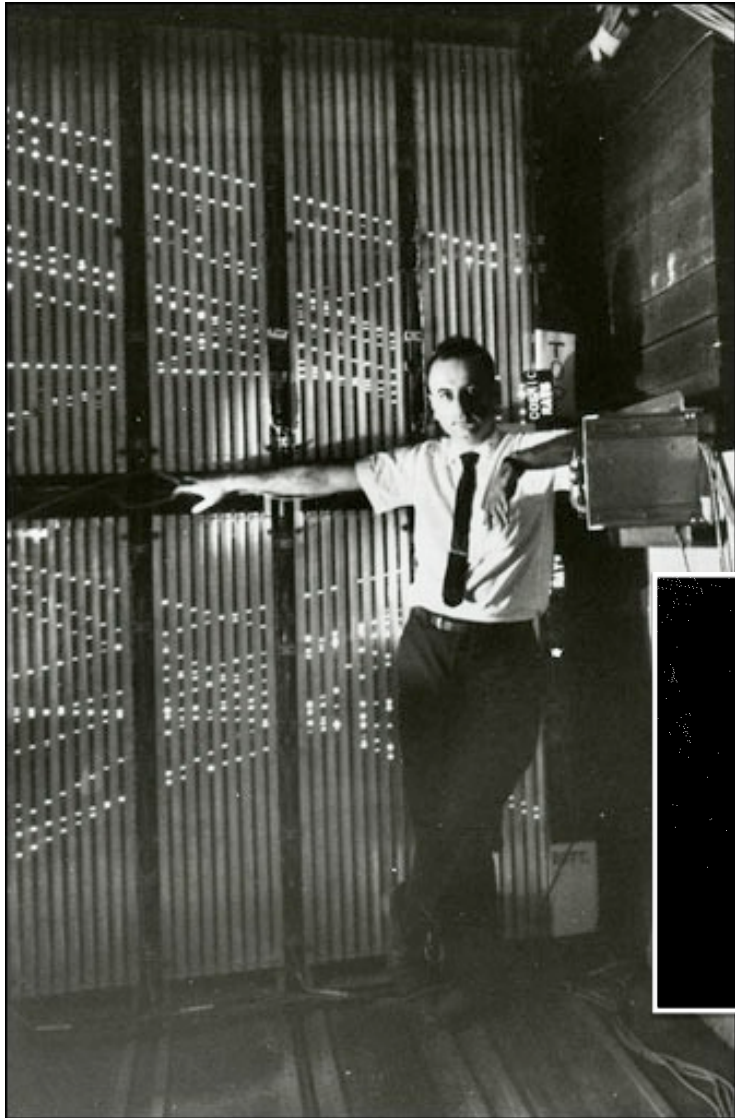
Melvin Schwartz in front of the spark chamber used to discover the muon neutrino
