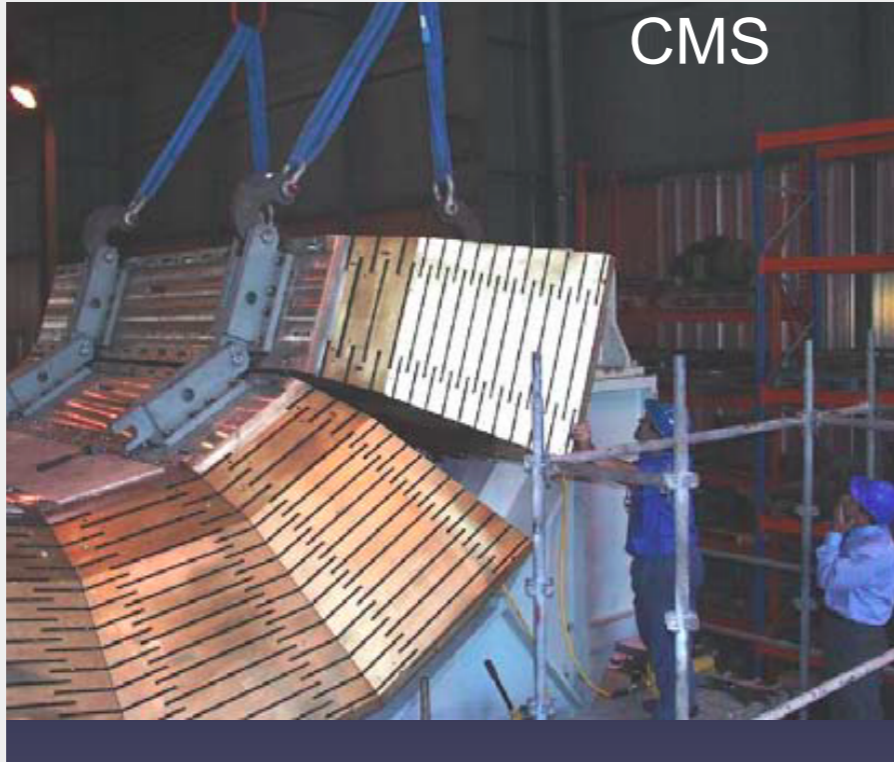
5 cm brass / 3.7 cm scint. Embedded fibres, HPD readout
