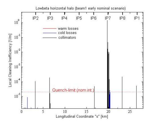
For this case only the aperture of TCTs and TCDQs is increased respectively from 8.30 to 170 and from 7.50 to 80. The losses on the cold aperture and on the collimators don't change significantly with respect to the nominal machine. Fort TCTs losses are even smaller and at IP5 there are no losses at all. The same behavior is found also for the vertical halo.
