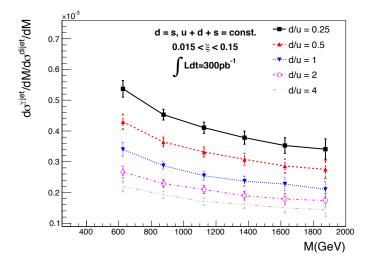
Taking into account the typical mass resolution around 3%, a significant measurement can be achieved with an integrated lumi of 300  $pb_{\pm}^{-1}$
