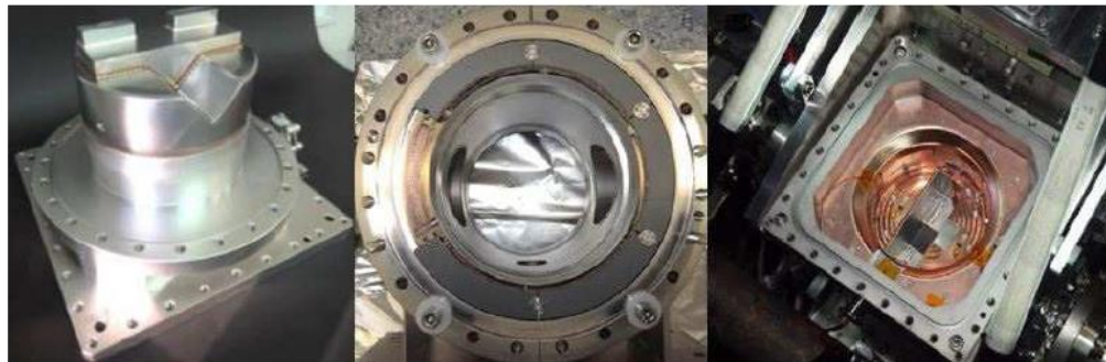
Fig. 9.3: Three of the main modifications implemented to minimise the effect of RF. From left to right: the RP filler with the copper contacts for proper grounding, the ferrites distributed as a ring on the flange of the station and the HDS (heat distribution system) in copper with the temperature probes attached to it.
