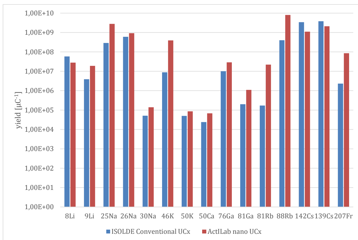
Figure 14: Preliminary results of the ActILab nano-structured \text{UC}_x (#525UC-Re) in comparison to conventional ISOLDE \text{UC}_x targets. The references are taken from the ISOLDE database; except for ^{26}\text{Na} and ^{88}\text{Rb} from measurements on targets #410 UC-W and #301UC-Ta.
