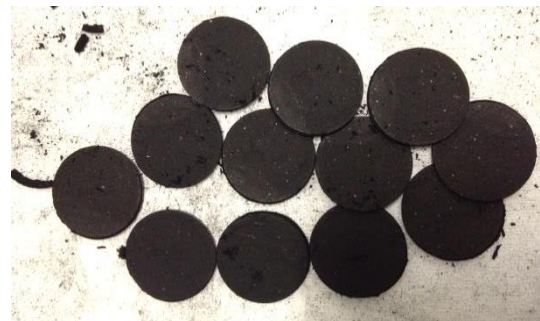
Figure 1 : reduced grain size distribution of the nano UO 2 versus the standard powder used, left. A set of pressed pellets used for a target nanoUC x load before online tests (14mm diameter), right.
