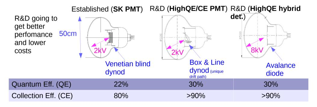
• It was finally decided to use the Box-and-Line (BL) high QE PMTs in the tank simulation, as suggested by the photosensors group.
