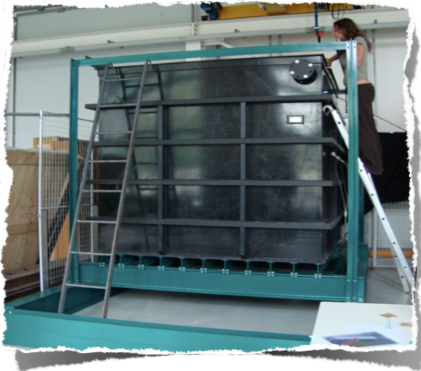
2x2x2 m 3 HDPE tank filled with filtered water
