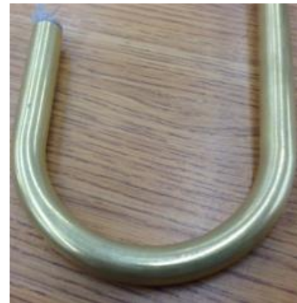
cable bent 180° on 2" radius.
