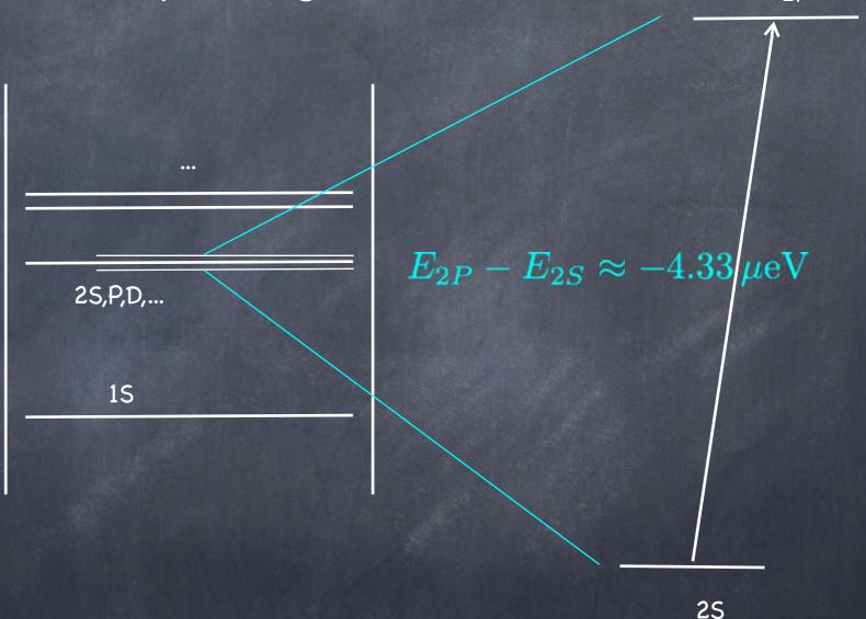
nS-nP splitting (Lamb shift) - authentic prediction of SM (QED) Precise calculations of QED corrections: p.p.m. level precision
