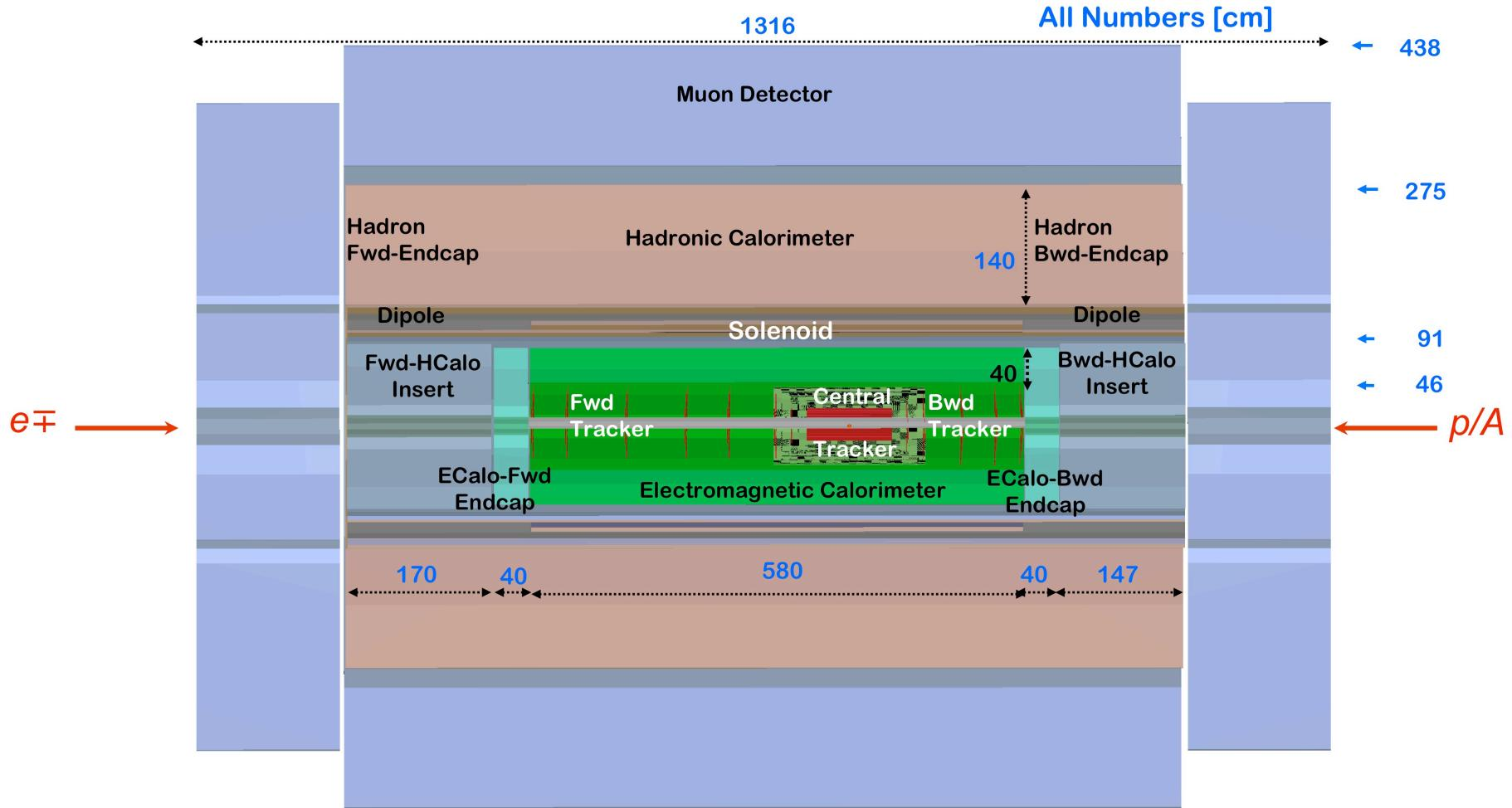
**Current (7/15) LHeC detector design** ( $14 * 9 \text{ m}^2$ , taggers (not shown), 3.5T solenoid
