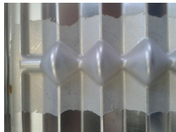
Sample with central part thinned to 150 \mu\text{m}
