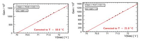
$\hookrightarrow$  Value of breakdown voltage is stable  $\leftrightarrow$ in considered temperature range of the measurements
