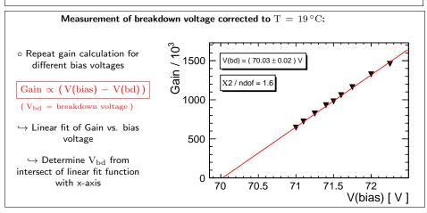
ECAL Lab Meeting | M. Munker | Gain and Breakdown Voltage Measurement for the used SiPM | p. 9
