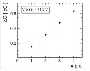
$\hookrightarrow$  Can calibrate measured charge to # p.e. with the measured gain:
