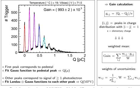
$\hookrightarrow \mbox{Check linear dependence of $Q(MPV) - Q(\mu)$ for different photoelectron peaks to validate calibration of charge to number of photoelectrons}$
