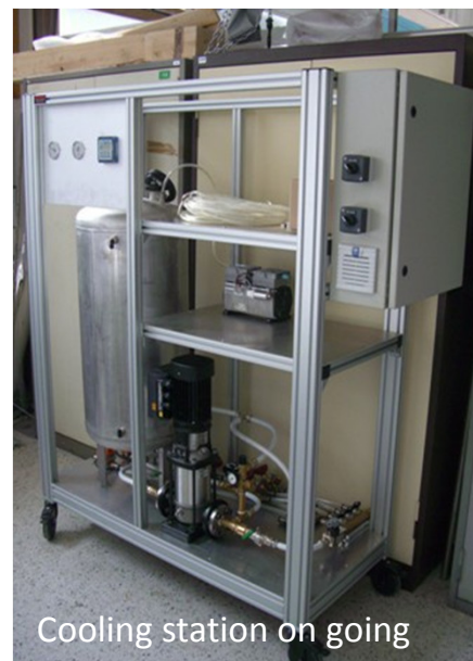
LPSC cooling test area with a drop of 13 m
